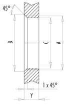
Installation direction: o-ring sits on chamfer.
